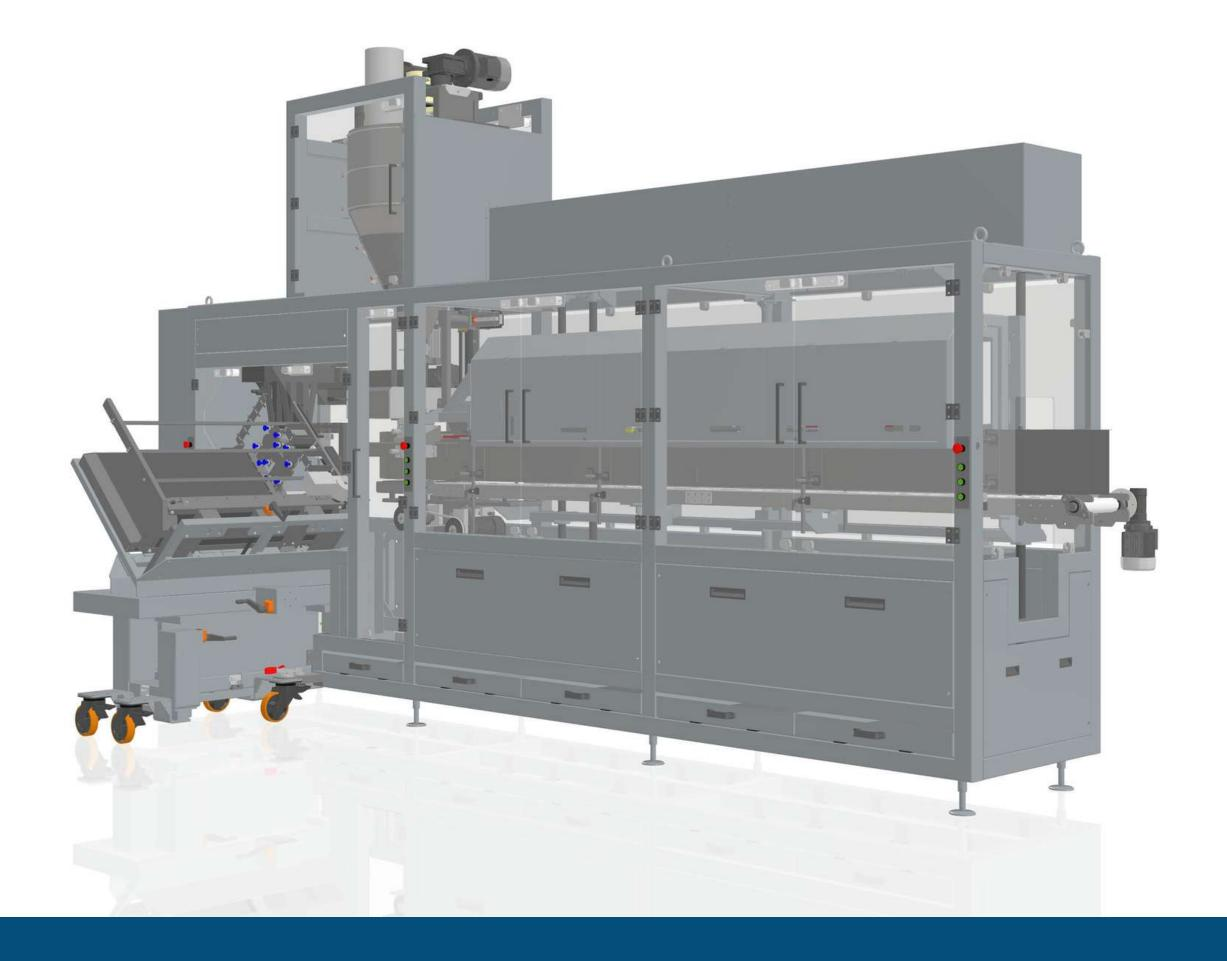
The C-10 packaging machine is a machine for chemical powders, such as additives and dyes, which allows an automatic format change in ten minutes and a wide range of adjustment for closing. It also features a double fin-fold bag closure with biodegradable watersoluble glue.
