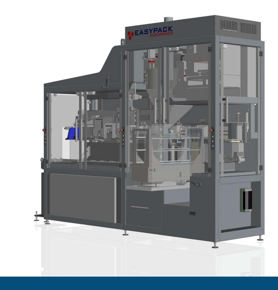
The B-20 packaging machine is a multi-format machine suitable for food powders and granules, which features a dual dosing system: by weight and volumetric and allows a format change in fifteen minutes. In addition, it features a single fin-fold bag closure with stitching.
