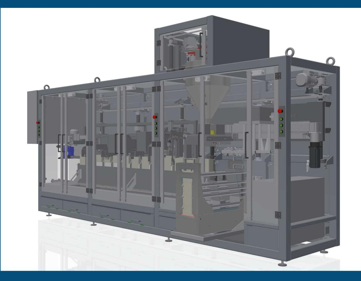
The B-30 packaging machine is a multiformat machine suitable for bagging food powders, allowing automatic format change in just fifteen minutes. It also features a double type of bag closure: double fin fold with stitching and hot melt glue.
